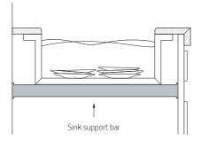
Furthermore, for large sinks, we recommend placing support bars under the sink, so that its weight is borne by the bars and not the worktop.
