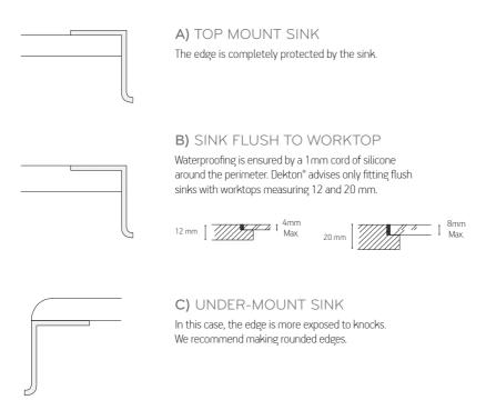
In this case, the edge is more exposed to knocks. We recommend making rounded edges. Sinks that include sloping surfaces must be made with a piece of the same material adhered on the underside with Mastidek; thus maintaining the original texture of the product. Below is an example of sink designs recommended by Dekton\*:
