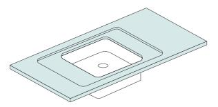
We do not recommend installing sinks of same material as the worktop and joined to the worktop with mitred edges as these do not respect the internal minimum radius of 5 mm.
