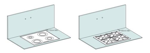
Dekton\* advises only fitting flush hobs with worktops measuring 12 and 20 mm, respecting the following distances:
