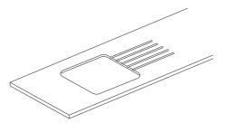
If the draining board is grooved, this part will require extra reinforcement.
