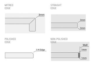
These edge type reduce the likelihood of chipping and breakage during use.
